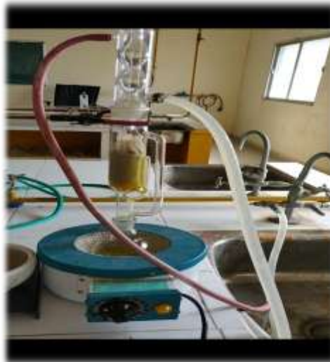
Fig 11: Soxhlet extraction of Brassica Nigra seeds
